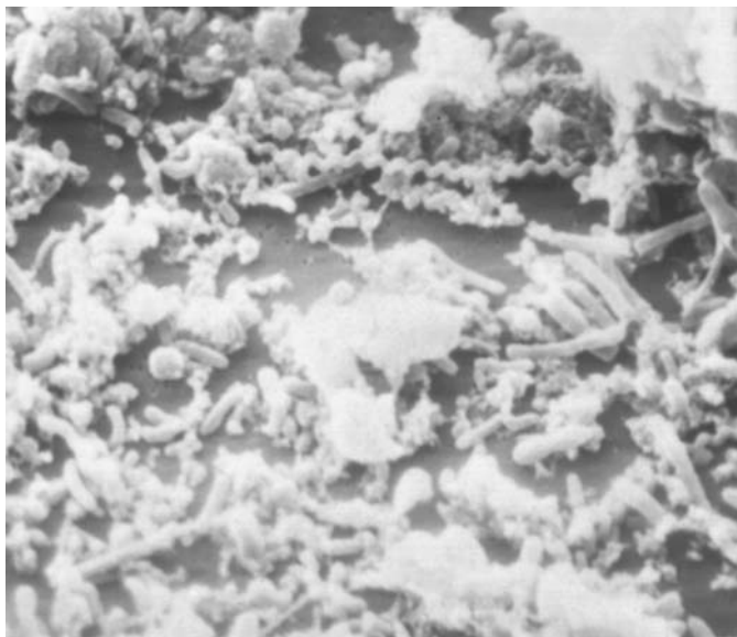
Figure 13.28 Gallionella -type bacteria causing iron precipitation in wells.
