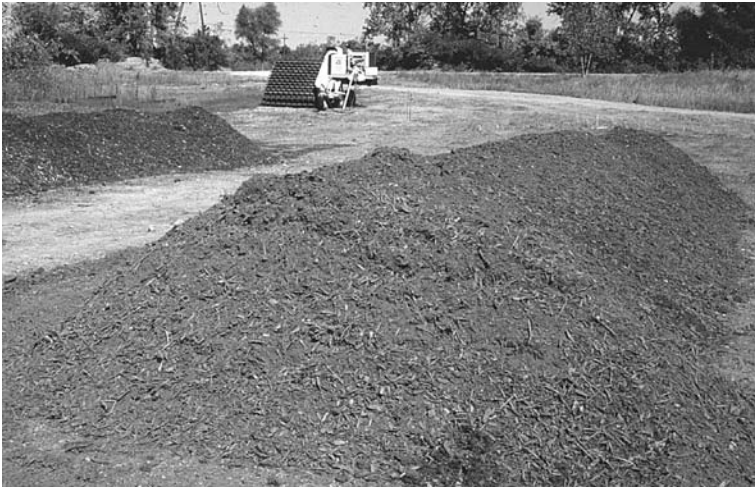
Figure 16.49 Windrow biosolids composting piles.
